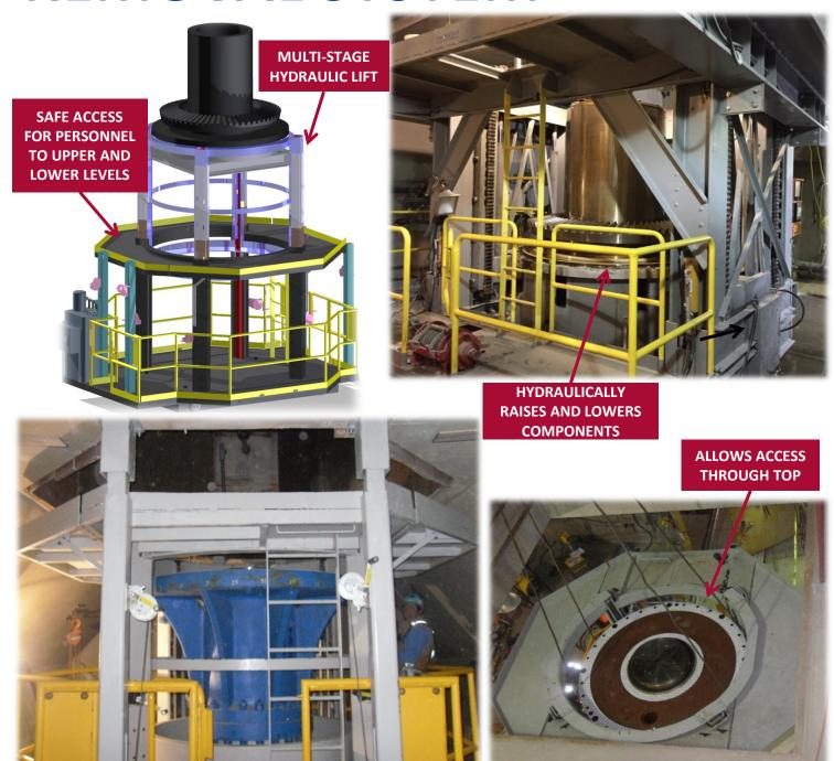
This cart is designed to eliminate rigging risks associated with the removal and replacement of the Hydroset and other eccentric components. This self powered cart positions itself under the crusher and provides bi-level access for personnel. The multi-stage hydraulic lift will raise to support the parts being replaced and safely lower them into the cart for transport. No need for cable slings!
